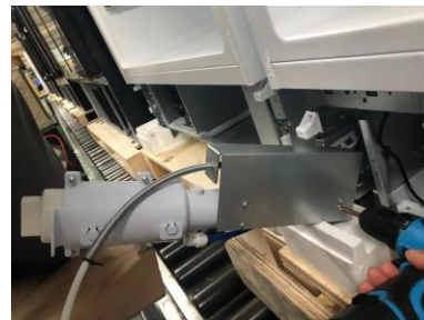
3. Remove the 2 screws holding the water valve
