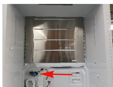
6. Water valve position in the tank
