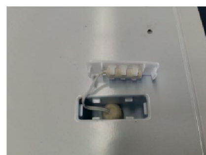
3. Open the ring temperature sensor
