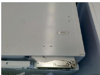
1. The case temperature sensor is located at the top of the refrigerator
