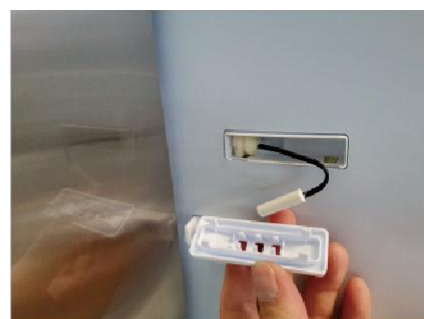
3. Separation of the lid from the sensor
