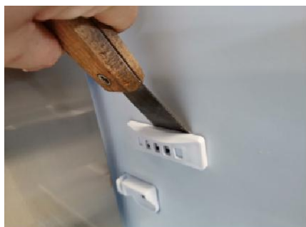
1. Use the flat shovel to pry open the box temperature sensor box cover
