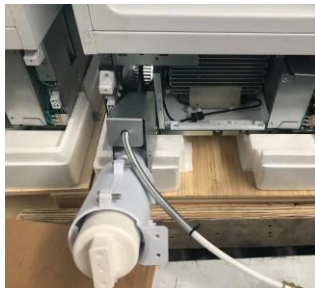
2. Pull out the filter and water valve
