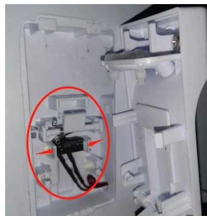
3. Carefully remove the microswitch
