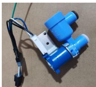
5. Unplug the terminal to remove the watervallve
