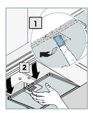
3. Press the tabs and push the LED bar outwards
