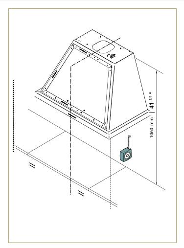
The fastening kit (screws and plugs) supplied with the hood can only be used on masonry wall. For installation on other types of walls consider alternative fastening systems, taking into a count the strength of the wall itself and the weight of the hood.
