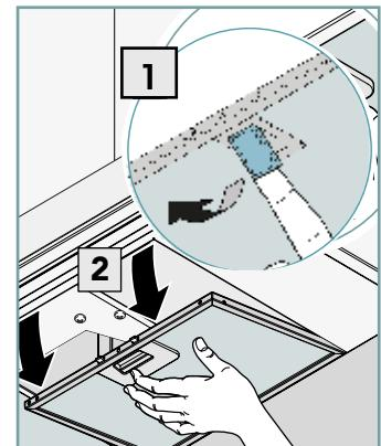
3. Press the tabs and push the LED bar outwards
