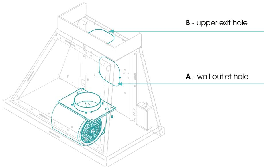
rotate the motor and fix
