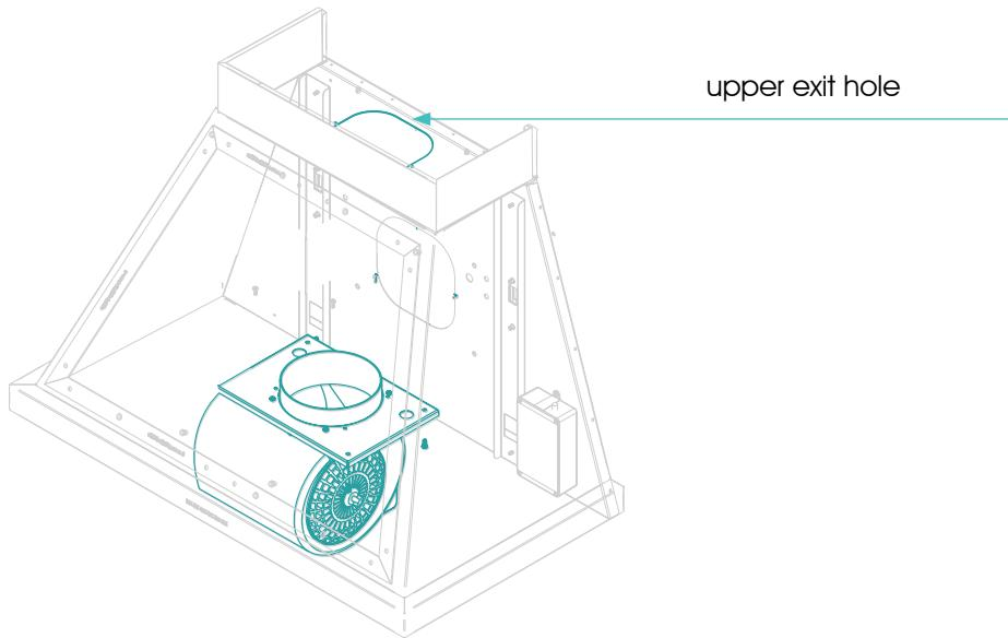
rotate the motor and fix
